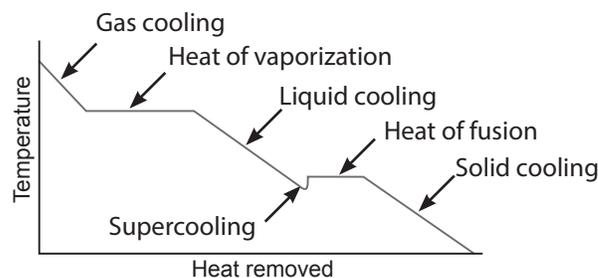
Supercooling is the cooling of a liquid below its freezing point without it becoming solid.
