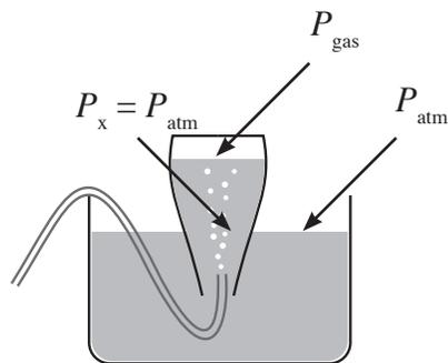
Because the pressure in a static fluid is the same everywhere at the same level,  $P_x$  must equal  $P_{\text{atm}}$ . Furthermore,  $P_x$  is at a greater depth in the fluid than the surface of the fluid in contact with the gas, which is at the same pressure as the gas. Therefore,  $P_x < P_{\text{gas}}$ .
