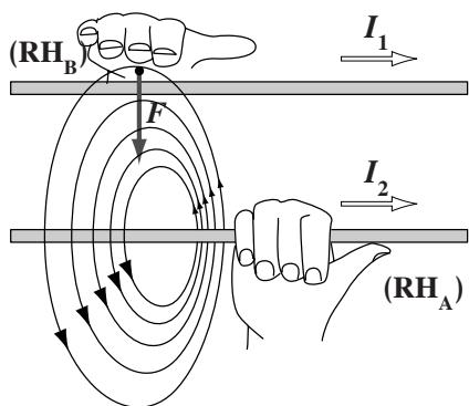
**RH<sub>A</sub>** – Point the thumb of your right hand in the direction of positive current, then wrap your fingers around the wire to show orientation of the magnetic field.
